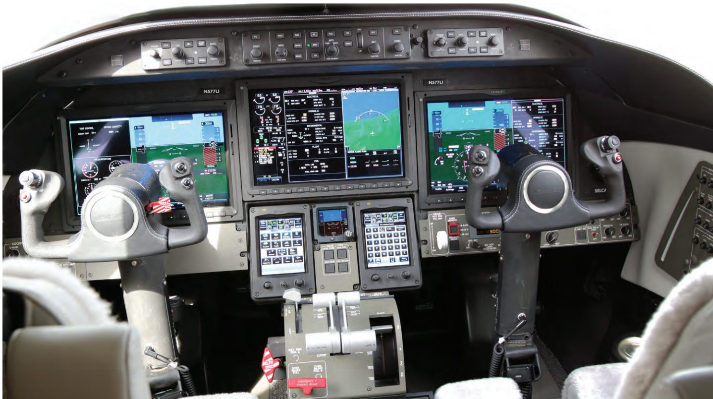
The cockpit of the Learjet 75 – certified to Part 25 standards, it features two independent Garmin 5000 flight control systems (pilot and copilot) with cross-over redundancies. (Photo by Hayden Hamilton)
