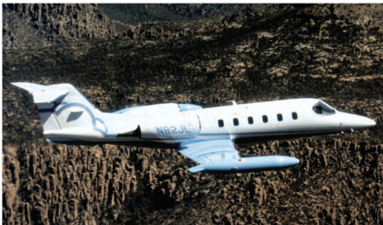
The Learjet 35 represented an upgrade of the 20-series with the engines being replaced with Garrett TFE731-2 turbofans, enhancing the range and service ceiling of the design. This model also saw service with the USAF designated as C-21A. (AAHS archives, AAHS-S052491)
