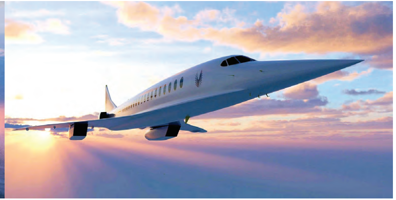
Boom Supersonic Overture supersonic transport designed to carry 65-85 passengers at Mach 2 plus. (Boom Supersonic photo)
