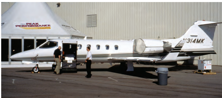
The Learjet 31 was a combination of the series 35 fuselage mated with the series 55 wings. Fitted with a glass cockpit and improved stability provided by the aft fuselage Delta-Fins offered higher performance with a maximum cruise altitude of 51,000 feet, rare even in today's market. (AAHS archives, AAHS-S052485)
